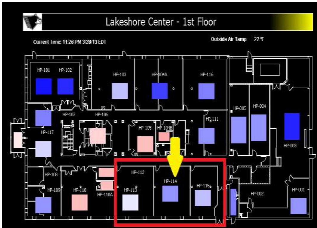
Figure 2.2: Layout of first floor of Lakeshore Centre showing all rooms and all heat pumps on that floor. [See Appendix C for documentation of permission to republish this material]
